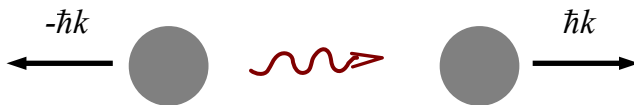
Figure 5: Photon reabsorption in an optically thick cloud. The photon emitted by the left atom can be reabsorbed by the right atom before leaving the atomic cloud. The recoil of the emitting atom is opposite to the recoil of the absorbing atom.
