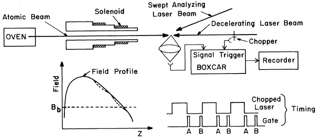
FIG. 1. Schematic diagram of apparatus including optical and electronic arrangement. A plot of  $B$  vs  $z$ , with and without the turns in the small shaded area of the solenoid, is shown. Note the regions of large  $dB/dz$  (steep slope on broken curve). The timing of the boxcar gates  $A$  and  $B$  relative to the chopping of the decelerating laser is shown at the lower right-hand side.
