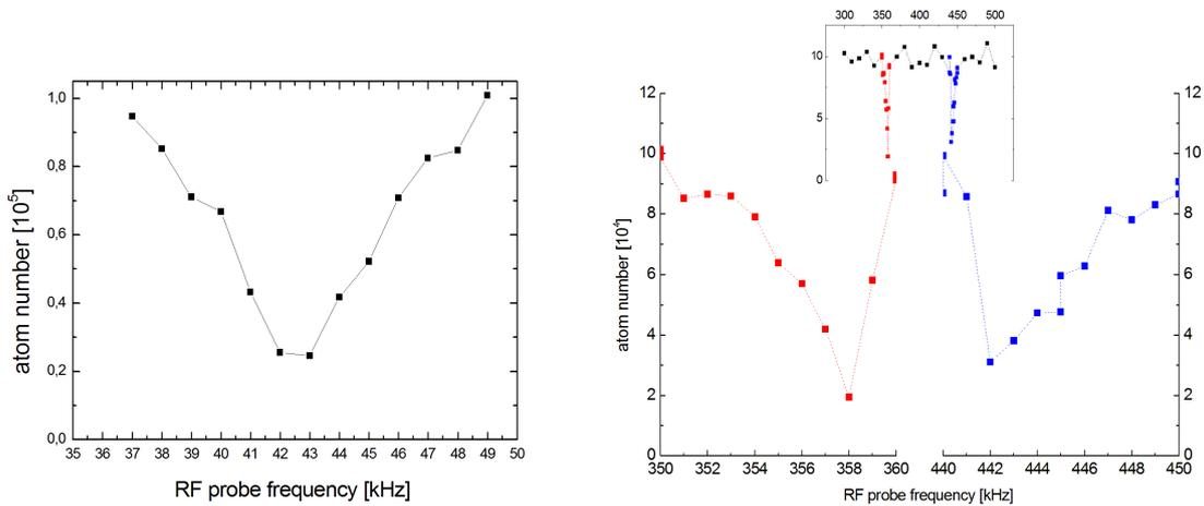
Figure 2: rf-spectroscopy of atoms confined in an adiabatic potential produced by a homogeneous rf field at frequency 400 kHz together with a quadrupole static magnetic field. Spin flips induced by a weak probe produce atom losses, which are recorded as a function of the probe frequency. Losses are observed around 42 kHz, 358 kHz and 442 kHz. Data taken at LPL.
